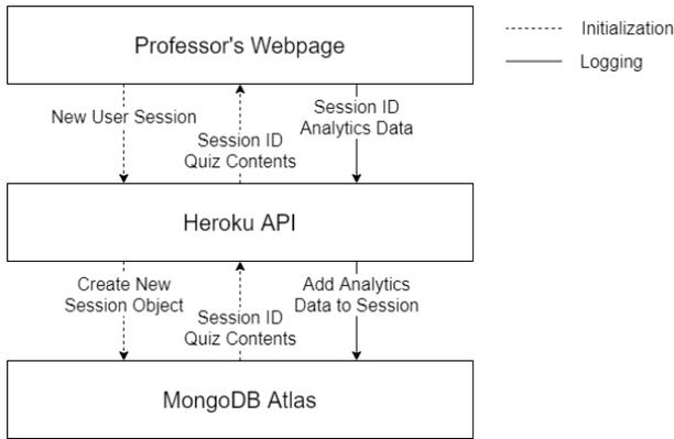
Fig. 4. Outline of the structure of the video logging system.
