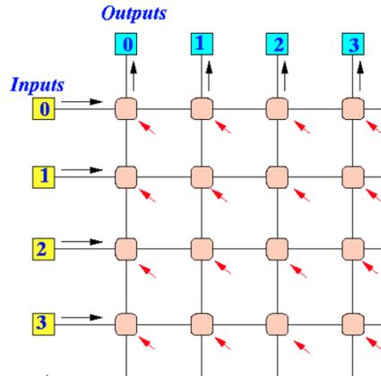
The crossbar implementation shown below uses a number of tri-state buffers located at the intersection point of each row and column to control the traffic.
