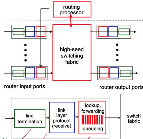
Figure 1. Router Architecture
