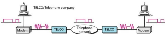
Figure 1: How Modems Communicate
