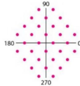
Figure 2: QAM Modulation
