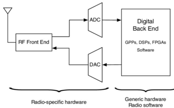
Figure 5: SDR Block Diagram
