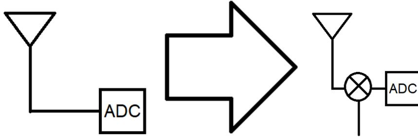
Figure 2: Circuit with and without mixer
