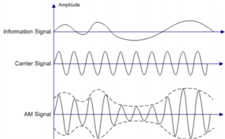
Figure 14: Amplitude Demodulation
