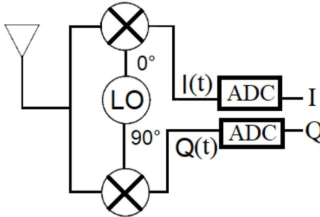
Figure 3: Circuit with two mixers
