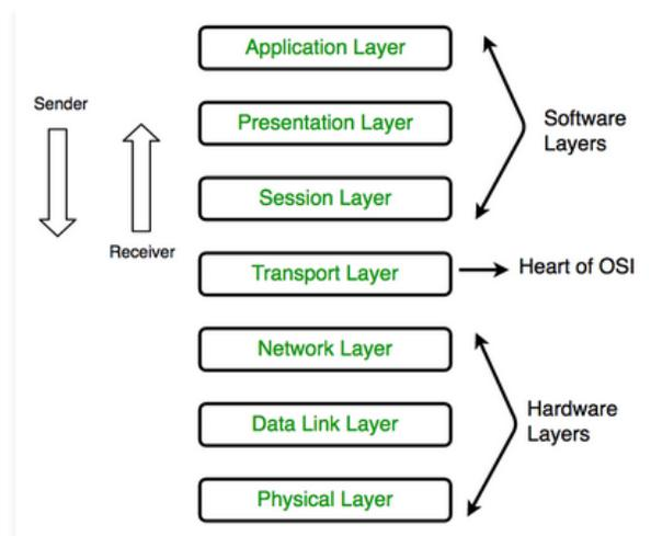
Figure 1: Layers of the OSI Model
