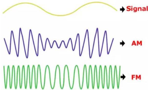
Figure 7: Amplitude Modulation and Frequency Modulation
