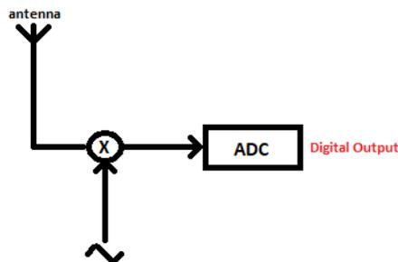
We can build a simple SDR that can pick up a wider range of signals using just our mixer and ADC. However, we can observe that the indistinguishability problem limits this design. Consider if an SDR of this design had:
