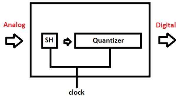
The sample holder converts the analog signal to a step function. Every cycle of its clock, it samples the signals amplitude and holds that value until its next cycle. The quantizer converts this held value to a digital value for output.
