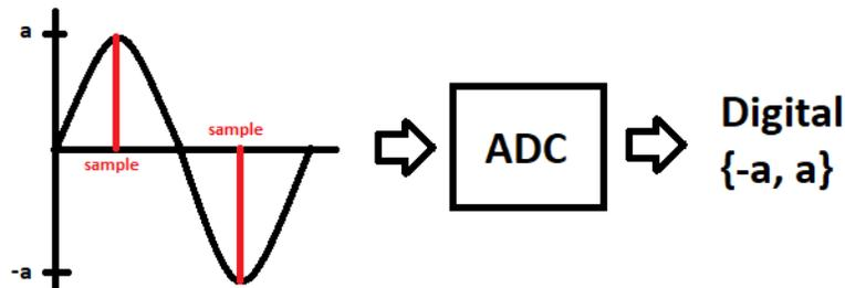
We must sample the signal through an analog digital converter (ADC) at a Hz at least twice its frequency to be able to reconstruct the wave.
